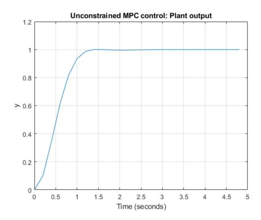
Running a closed-loop simulation in which all controller constraints are turned off is easier using sim, as you just need to specify 'off' in the Constraint field of the related mpcsimopt simulation option object.
