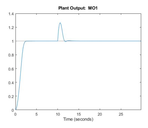
In an effort to reject the measured disturbance, achieve tracking, and prevent the output from rising above its soft constraint of 1.1, the controller slightly violates the soft constraint on the manipulated variable, which reaches small negative values from seconds 10 to 11. The controller violates the constraint on the measured output more than the constraint on the manipulated variable.
