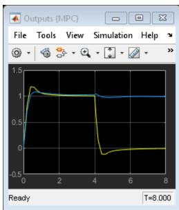
The inputs and outputs signals look identical for both loops. Also note that the manipulated variable are no longer bounded by the previous constraints.
