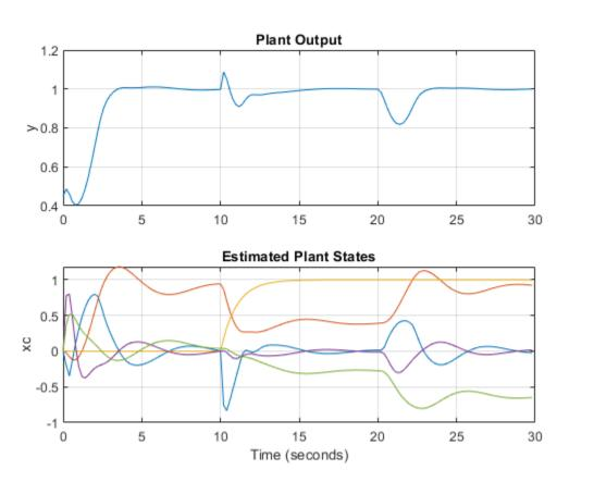
As expected, the measured and unmeasured disturbances cause sudden changes at 10 and 20 seconds, respectively.
