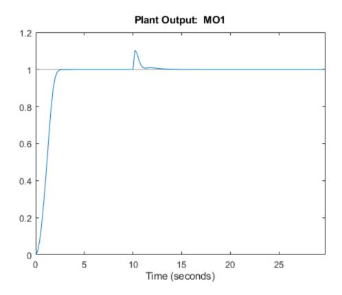
Now the controller violates the output constraint only slightly. This output performance improvement comes at the cost of violating the manipulated variable constraint a lot more (the manipulated variable reaches a value of -3).
