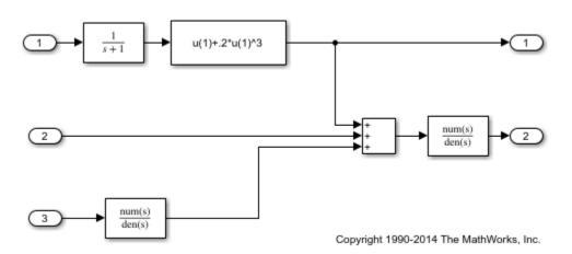
Linearize the plant at the default operating conditions (the initial states of the transfer function blocks are all zero) using the linearize command from the Simulink Control Design Toolbox.
