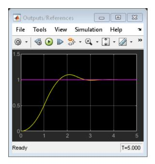
The closed-loop response shows good setpoint tracking performance, as the plant output tracks its reference after about 2.5 seconds. As expected, the manipulated variable stays within the predefined constraints.
