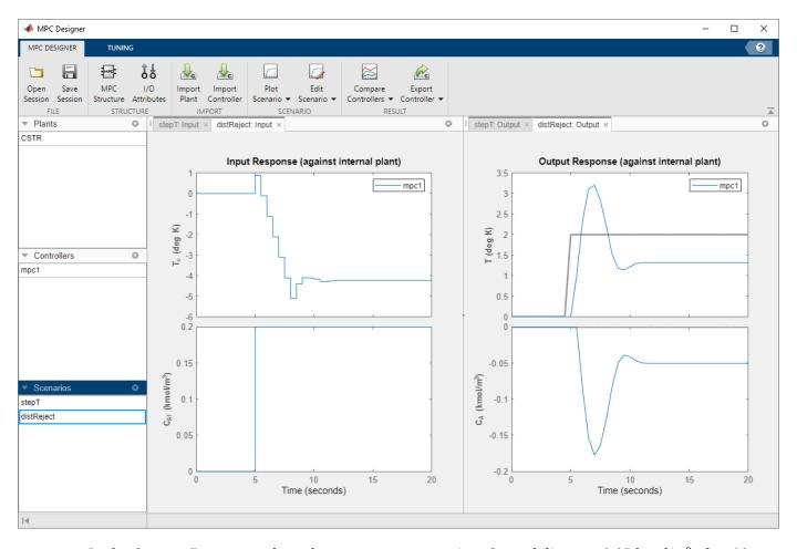
In the **Output Response** plots, the reactor concentration,  $C_A$ , stabilizes at -0.05 kmol/m³ after 10 seconds. Since there is only one manipulated variable, the controller makes a compromise between the two competing control objectives: Temperature tracking and constraint satisfaction. A softer output constraint enables the controller to sacrifice the constraint requirement more to improve the temperature tracking.
