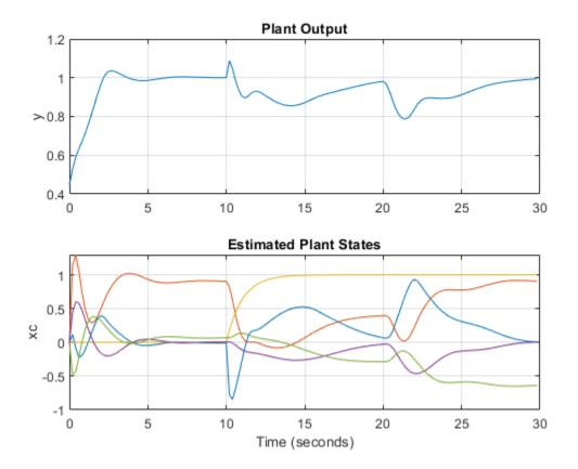
As expected, the controller states are different from the ones previously plotted, and the overall closed-loop response is somewhat slower.
