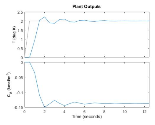
The plant/model mismatch degrades the controller performance, as you can tell from the oscillatory behavior of the closed loop responses. Degradation can be severe and must be tested on a case-by-case basis.
