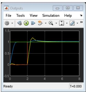
Despite the presence of the nonlinearity, both outputs track their references well after a few seconds, while, as expected, the manipulated variables stay within the preset hard constraints.
