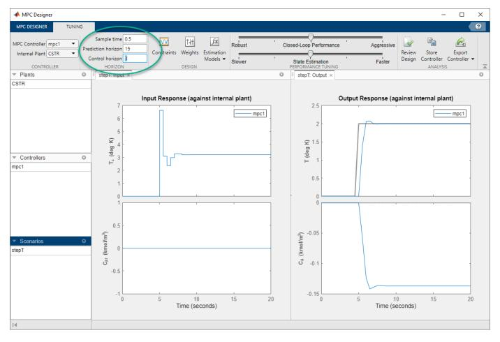
The response plots update to reflect the new horizons. The **Input Response** plot shows that the control actions violate the required constraint on the rate of change for the coolant temperature.
