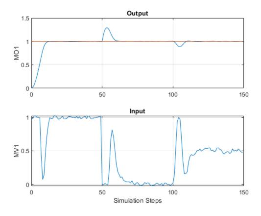
Despite the added noise, which is especially visible on the manipulated variable plot, and despite the measured and unmeasured disturbances starting after 50 and 100 steps, respectively, the controller is able to achieve good tracking. The manipulated variable settles at about 1 after the initial part of the simulation (steps from 20 to 50), at about 0 to reject the measured disturbance (steps from 70 to 100), and at about 0.5 to reject both disturbances (steps from 120 to 150).
