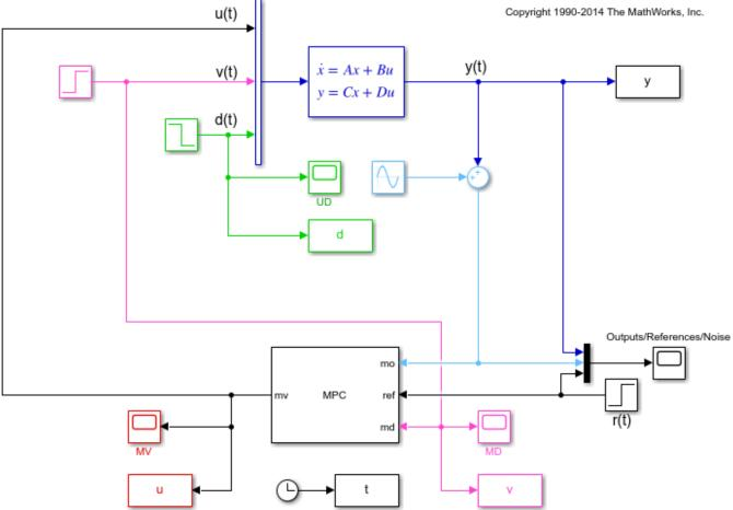
Since this noise is expected, you can specify a noise model to help the state estimator ignore it. Doing so improves the disturbance rejection capabilities of the controller.
