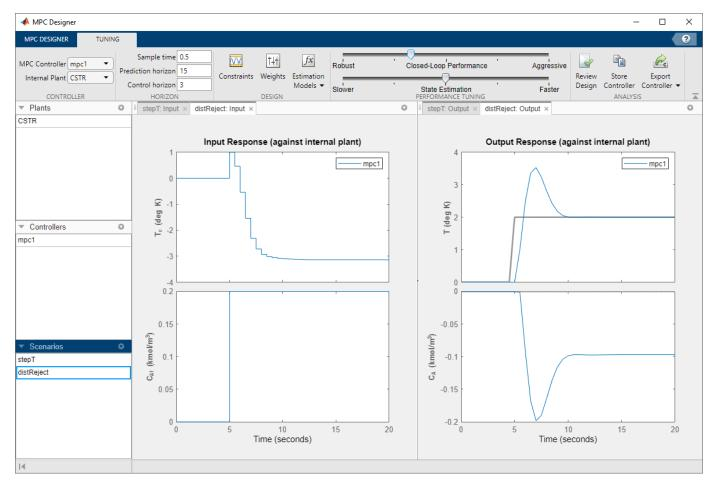
As you can see from the **Output Response** plots, the closed-loop system is still able to reach the desired reactor temperature. In this case, the required control actions, combined with the input disturbance, cause a steady-state decrease in the output concentration,  $C_A$  of 0.1 kmol/m<sup>3</sup>.
