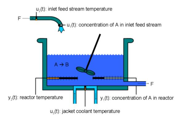
The inputs of the CSTR model are arranged in the vector u(t) and are as follows.
