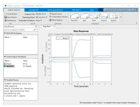
The step response from feed concentration to output CSTR/2 displays an interesting inverse response. An examination of the linear model shows that CSTR/2 is the residual CSTR concentration,
