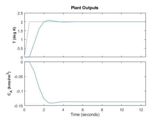
The first move of the manipulated variable now exceeds the specified 1-unit rate constraint.
