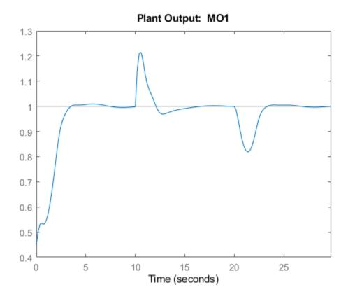
As a result of the model mismatch, some degradation in the response is visible; notably, the controller needs a little more time to achieve tracking and the manipulated variable now settles at about 0.5 to reject the measured disturbance (see values from 5 to 10 seconds) and settles at about 0.9 to reject both input disturbances (from 25 to 30 seconds). Despite this degradation, the controller is still able to track the output reference.
