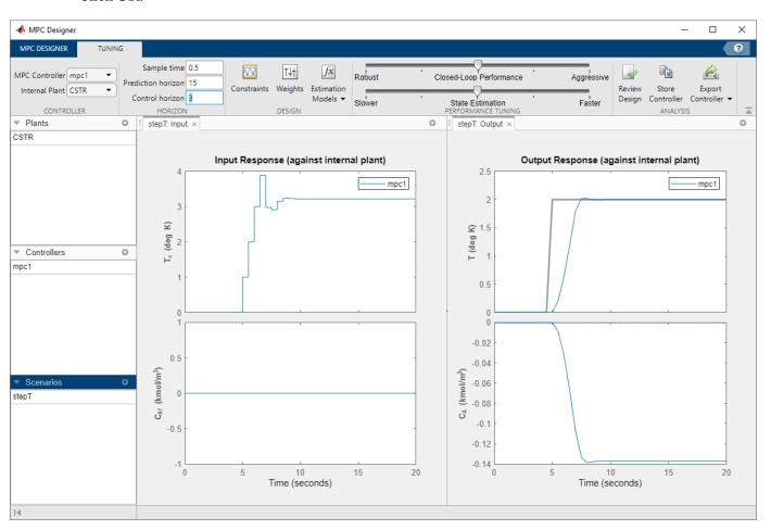
The **Input Response** plot shows the constrained manipulated variable control actions.
